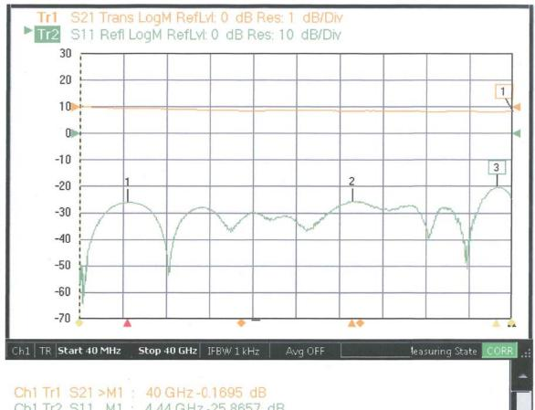
Ch1 Tr1 S21 >M1 : 40 GHz -0.1695 dB Ch1 Tr2 S11 M1 : 4.44 GHz -25.8657 dB Ch1 Tr2 S11 M2 : 25.16 GHz -25.5073 dB Ch1 Tr2 S11 >M3 : 38.56 GHz -20.2706 dB
